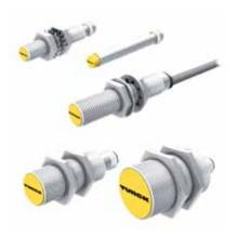
Typical applications for magnetic-inductive sensors include "pig" detection and gate monitoring. Since magnetic-inductive sensors are actuated by external magnetic fields, they achieve large switching distances despite their small size. In combination with the actuation magnet DMR31-15-5, the M12 sensors attain a rated switching distance of 90
