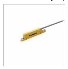
General data Measuring range 45 mm **Protection class** IP67 Operating voltage 15...30 VDC Output Analog output, 4...20 mA, 0...10 V **Housing material** PA12-GF30 **Ambient temperature** -25...+70°C Dimensions 5 x 14.5 x 73 mm Repeatability 0.1% of measuring range IA - BI
